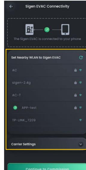
If the WLAN hotspot at the owner's premises is connected or if the SIM card APN is set (the device has a SIM card installed), click "Finished" to go to the page for creating new systems. You can refer to the description in the "already connected to the internet" section
