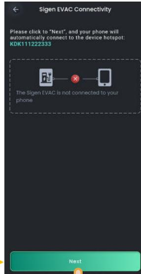
Connect to the equipment's WLAN hotspot. The hotspot is named as equipment SN and the passcode is given on the UI.
