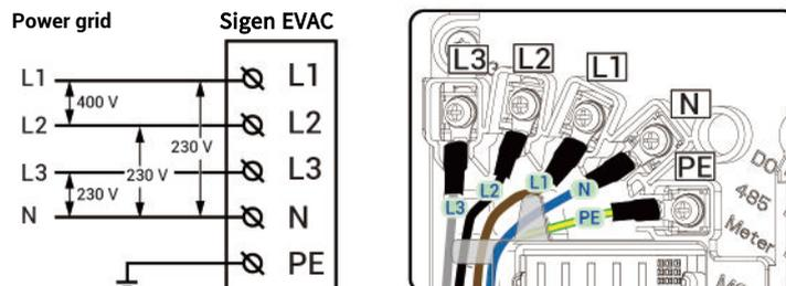
Three-phase four-wire system (L1/L2/L3/PE)
