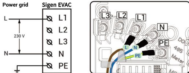
Three-phase five-wire system (L1/L2/L3/N/PE)
