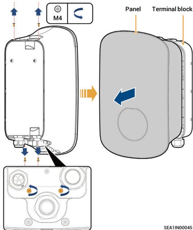
**3** Install and secure the terminal block.
